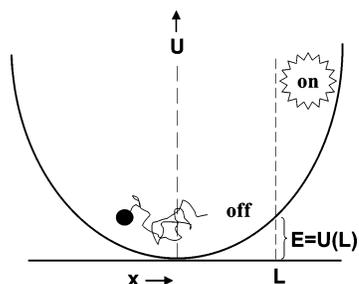
**Figure 1.** Illustration of the model of intermittency introduced in section II. The black circle is a particle moving stochastically in a harmonic potential well. The distance,  $L$ , is a critical control parameter (see the text for details.)
