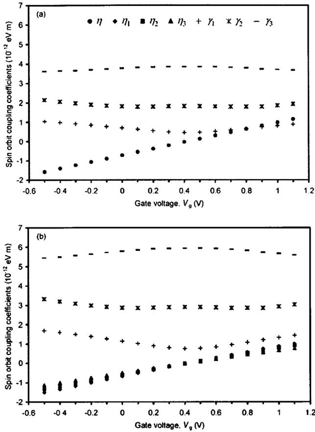
FIG. 2. Rashba,  $\eta_i$  and Dresselhaus,  $\gamma_i$ , spin-orbit coupling coefficients as a function of the gate voltage. Indexes correspond to different subbands. (a) Case I: phenomenological parameters fitted to experimental data (Ref. 27), (b) Case II: parameters calculated according to Ref. 40.
