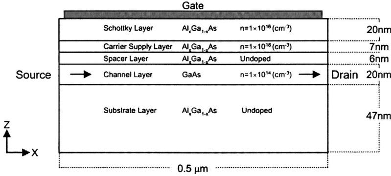
FIG. 1. Schematic diagram of the structure simulated,  $x=0.3$ .
