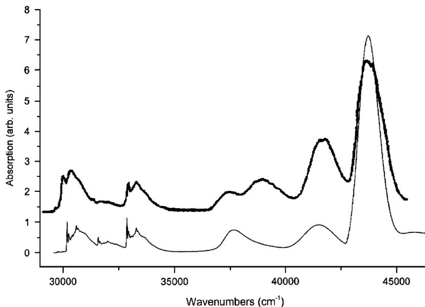
Fig. 3. Simulated (lower curve) and measured ( $T = 8$  K) [20] (upper curve)  $\sigma$ -polarized absorption from the lowest crystal field sublevel of the  ${}^1D_2$  multiplet in  $\text{LiYF}_4:\text{Pr}^{3+}$ .
