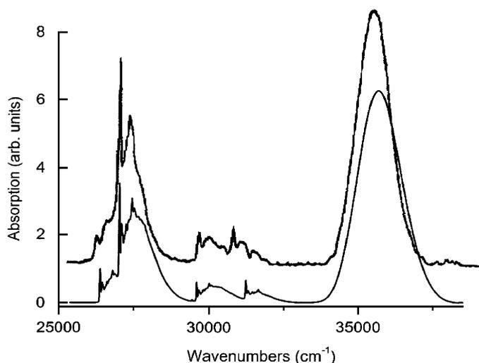
Fig. 6. Simulated (lower curve) and measured ( $T = 8$  K) [20] (upper curve)  $\pi$ -polarized absorption from the  $^3P_0$  state of  $\text{Pr}^{3+}$  in  $\text{LiYF}_4$ .
