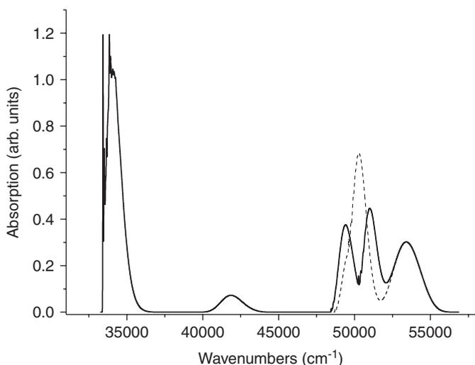
Fig. 1. Simulated unpolarized absorption in  $\text{LiYF}_4:\text{Ce}^{3+}$  at  $T = 0$ . The dashed envelope was obtained without taking into account the interaction with the non-adiabatic phonons.
