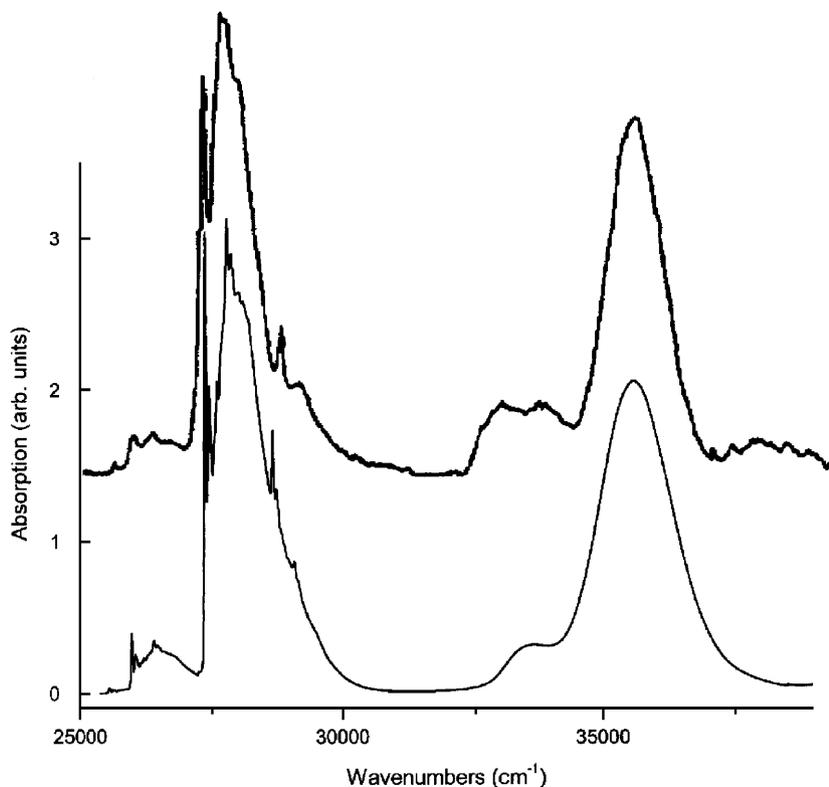
Fig. 5. Simulated (lower curve) and measured ( $T = 8$  K) [20] (upper curve)  $\sigma$ -polarized absorption from the  $^3P_0$  state of  $\text{Pr}^{3+}$  in  $\text{LiYF}_4$ .
