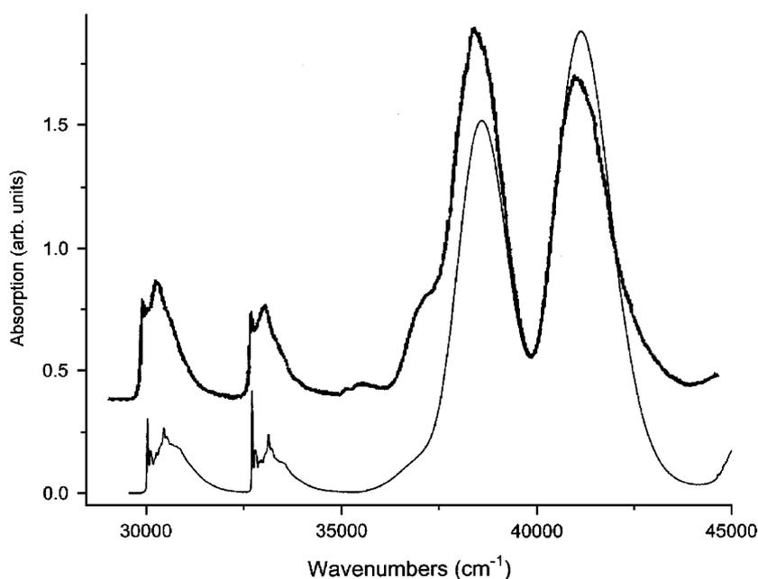
Fig. 4. Simulated (lower curve) and measured ( $T = 8$  K) [20] (upper curve)  $\pi$ -polarized absorption from the lowest crystal field sublevel of the  ${}^1D_2$  multiplet in  $\text{LiYF}_4:\text{Pr}^{3+}$ .
