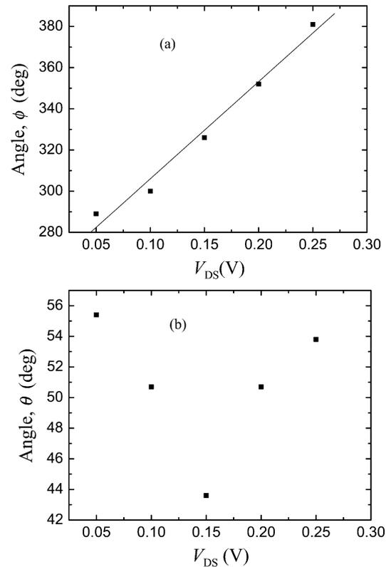
Fig. 5. Orientation of the spin polarization vector at the drain boundary at  $T = 77$  K. The angle  $\phi$  is measured in the  $xz$  plane, from the  $x$  axis, and  $\theta$  is measured in the  $yz$  plane, from the  $y$  axis. ( $\xi = 0$ ).
