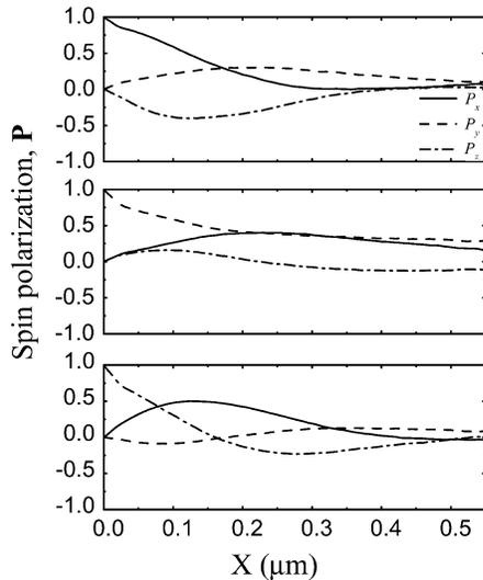
Fig. 4. Evolution of spin polarization for three different injected orientations. The device channel is parallel to the  $(1, 0, 0)$  crystallographic direction ( $\xi = 0$ ).  $T = 300$  K and  $V_{DS} = 0.1$  V.
