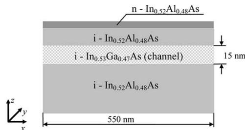
Fig. 1. Device structure for the simulations.
