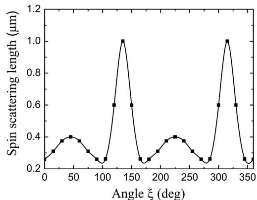
Fig. 6. Angular dependence of spin scattering length. Injected spin polarization is parallel to the device channel.  $T = 300$  K and  $V_{DS} = 0.1$  V.
