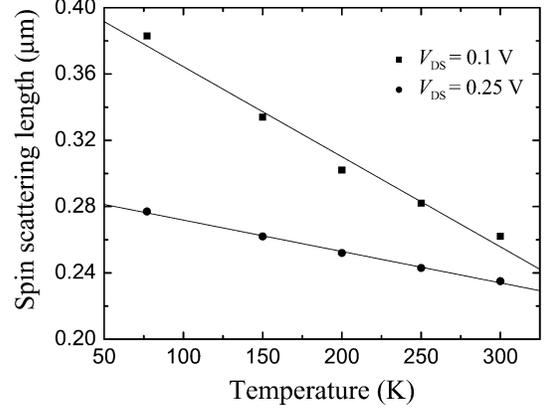
Fig. 3. Spin scattering length as a function of temperature. The device channel is oriented parallel to the (1, 0, 0) crystallographic direction. Injected spin polarization is in the channel direction.
