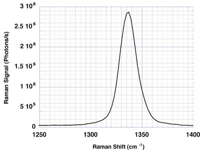
Fig. 5. Raman spectrum of a 0.9-mm thick (111) diamond obtained with 30 mW of 1064-nm excitation and 1.0-s integration time.
