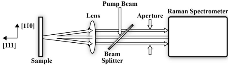
**Fig. 1.** Schematic of the optical setup for the measurement of Raman cross section; the sample is located in the focal plane of a 20-mm effective focal length (EFL) lens.
