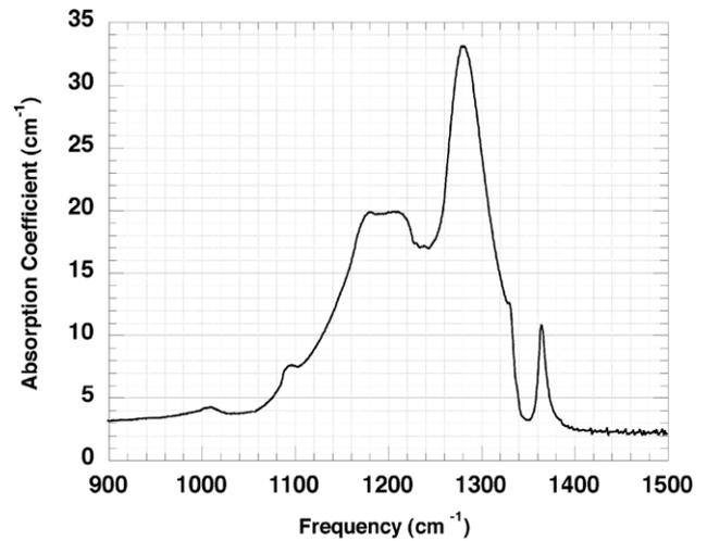
Fig. 3. IR absorption spectrum of the 0.9-mm thick (111) diamond sample obtained with a spectral resolution of  $2 \text{ cm}^{-1}$  using Fourier transform infrared (FTIR) spectrometer Nicolet 4700.
