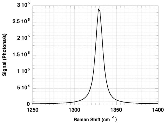
Fig. 4. Raman spectrum of a 0.9-mm thick (111) diamond obtained with 1.0 mW of 785-nm excitation and 1.0-s integration time.
