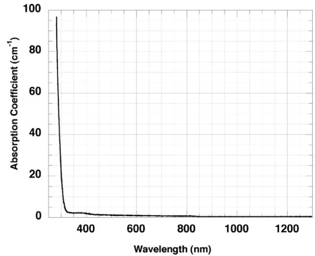
Fig. 2. UV–V–NIR absorption spectrum of the 0.9-mm thick (111) diamond sample obtained using Perkin–Elmer spectrometer 950.
