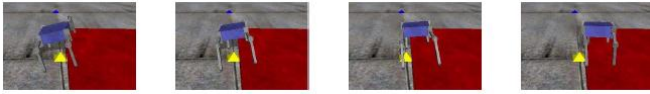
Fig. 3. Simulated robot executing a sequence of controls to climb up a single 4 cm step.
